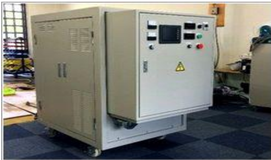
EcoEne Gas System KJC-2014-70h [Fuel supply amount Maximum 150L/h specifications]
